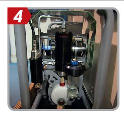
it is not enough to disturb the whole household. A quick check with a decibel app shows a working volume of 82dB at 2 foot, and 72 dB from 8 feet away. The footprint of the compressor is surprisingly small. I have it on a little stand just in front of the back door to keep it cool when in use, but tucked out of the way under a coat rack. Dimensions are: 18¼ inch (46.3 cm) by 9 inch (22.8cm) by 15 inch (38.1cm).
